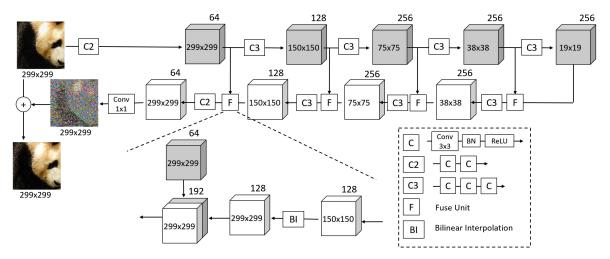
Figure 3: The detail of DUNET. The numbers inside each cube stand for width  $\times$  height, and the number outside the cube stands for the number of channels. In all the C3 of the feedforward path, the stride of the first C is  $2 \times 2$ .
