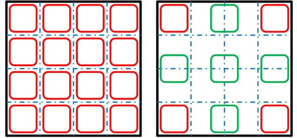
**Fig. 2.** An example of original (left) and sparser (right) spatial pooling in the 2nd layer (pooling bin size is  $\frac{W}{4} \times \frac{H}{4}$ ). We set  $s_2 = 3$ , so that some regions on the image plane are not occupied by any one of the pooling bins.
